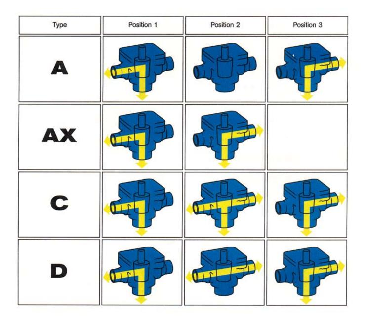
All of the valves shown in this catalogue can be supplied in a three way form. In order to achieve the required flow configuration one of the above plug types is required to be fitted in the valve.
