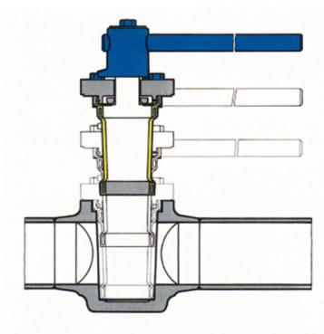
The **Easi-Sleeve** incorporates all the advantages of the established TUFLIN sleeved plug valve such as:
